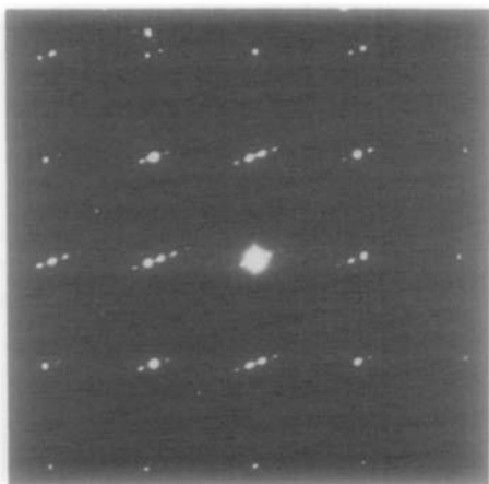
FIG. 3. Electron diffraction pattern taken of a transported crystal fragment with n \sim 24 . The diffraction spots are somewhat streaked which indicates disorder.
